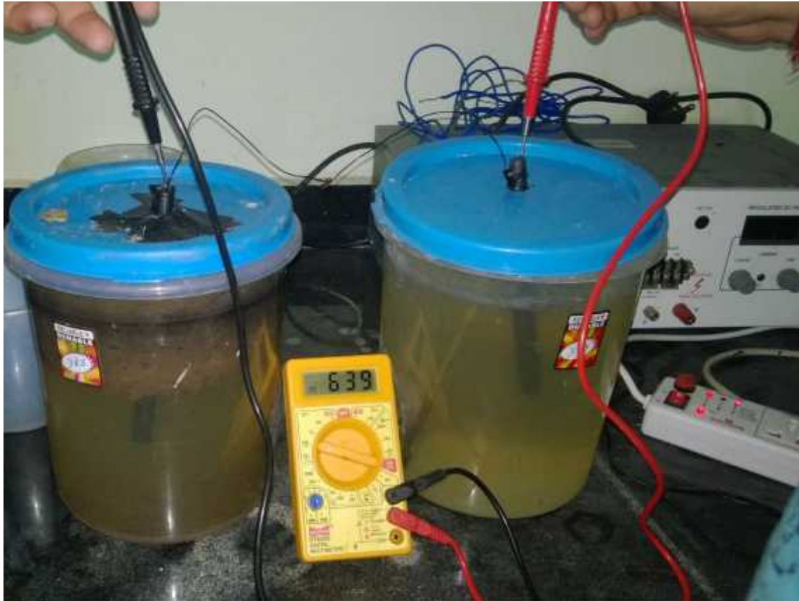
Fig. 4 - Peak value of OCV with secondary clarifier sludge as cathodic chamber and tap water aerator as an anodic chamber.
