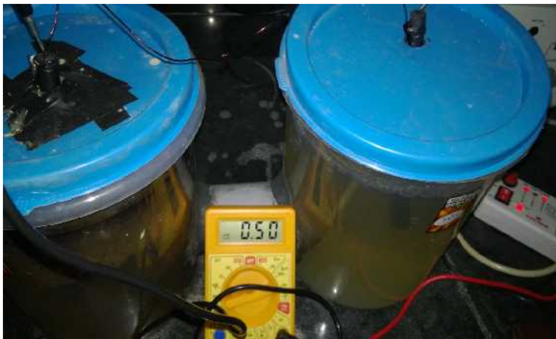
Fig. 5 - Peak value of OCV with secondary clarifier sludge as cathodic chamber and tap water aerator as an anodic chamber.
