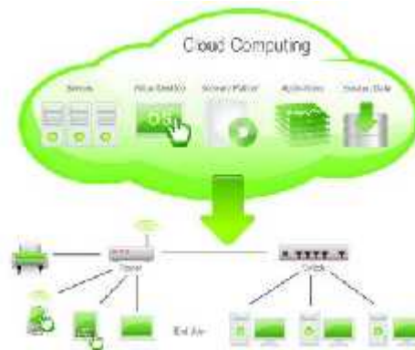
Figure 3: Working Principle of Cloud Computing
